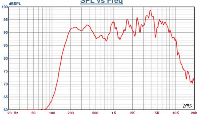
Sound pressure levels at 1W/1m w/P-4x6 closed SPL vs Freq
